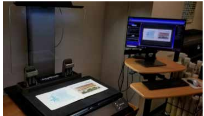
Scanning technicians use a special scanner to digitize books and other thicker media
